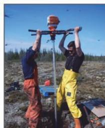
1. Permafrost drilling with core recovery
